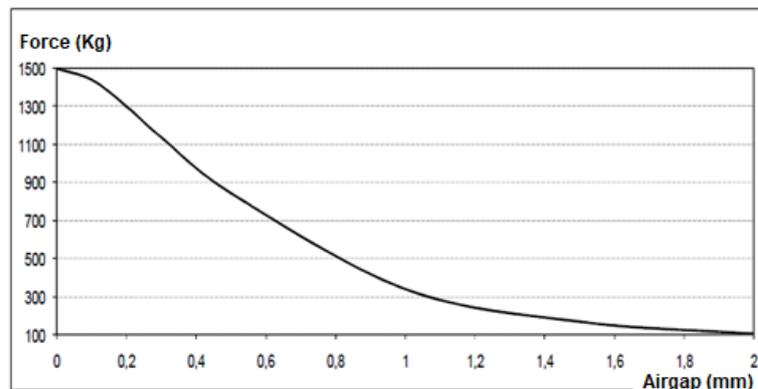
**IMPORTANT**, when used to lift pieces, apply a safety factor 3. The weight of the load must be less than 3 times the force of detachment.
