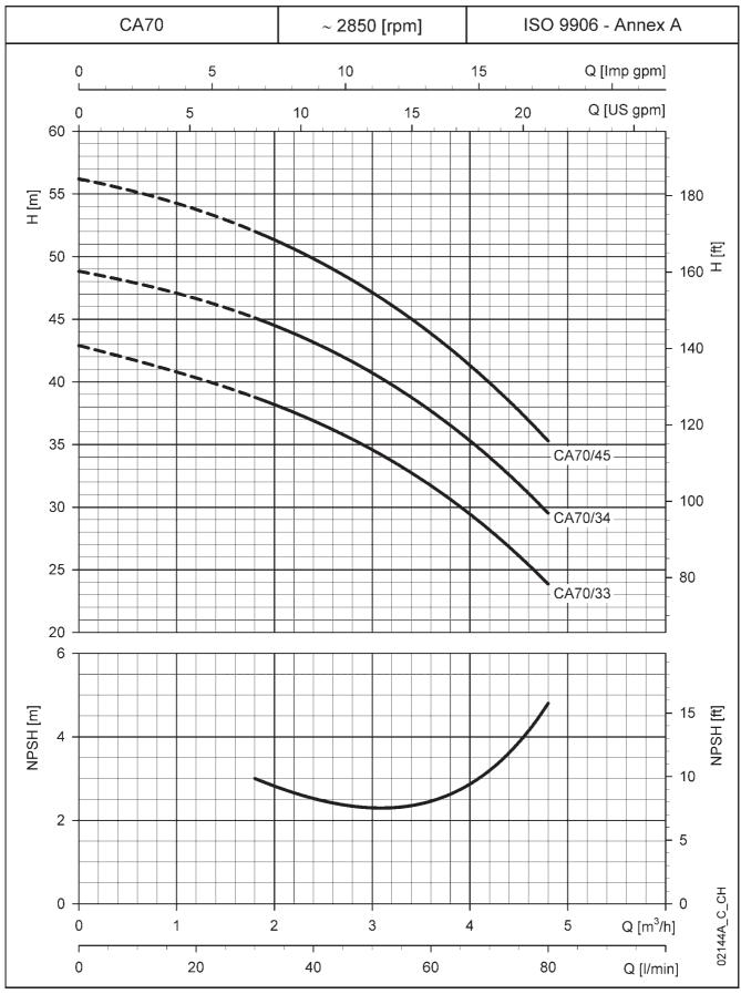
These performances are valid for liquids with density  $\rho=1.0~\text{Kg/dm}^3$  and kinematic viscosity  $\nu=1~\text{mm}^2/\text{sec.}$
